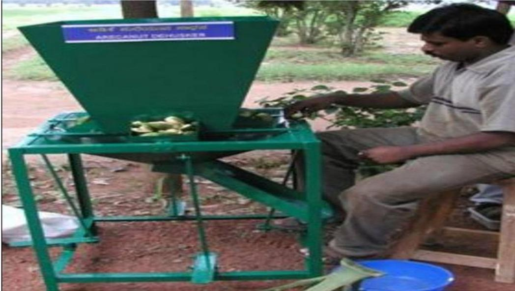
*Gambar. .4 Alat Pengupas Model Pedal*
